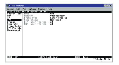
Figure 4-4. Configuration/IPX Screen
